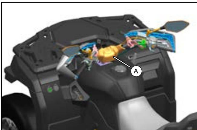
// Remove the steering handlebar cover (A).
